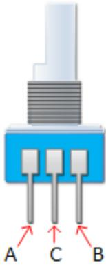
On one side of the switch there are three pins. They are normally referred to as A, B and C. In the case of the KY-040, they are oriented as shown.
