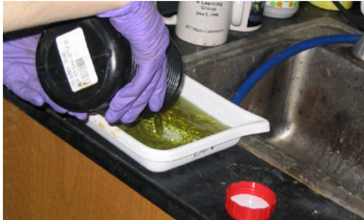
Carefully pour into a tray. The developer is green from use, it starts out clear
